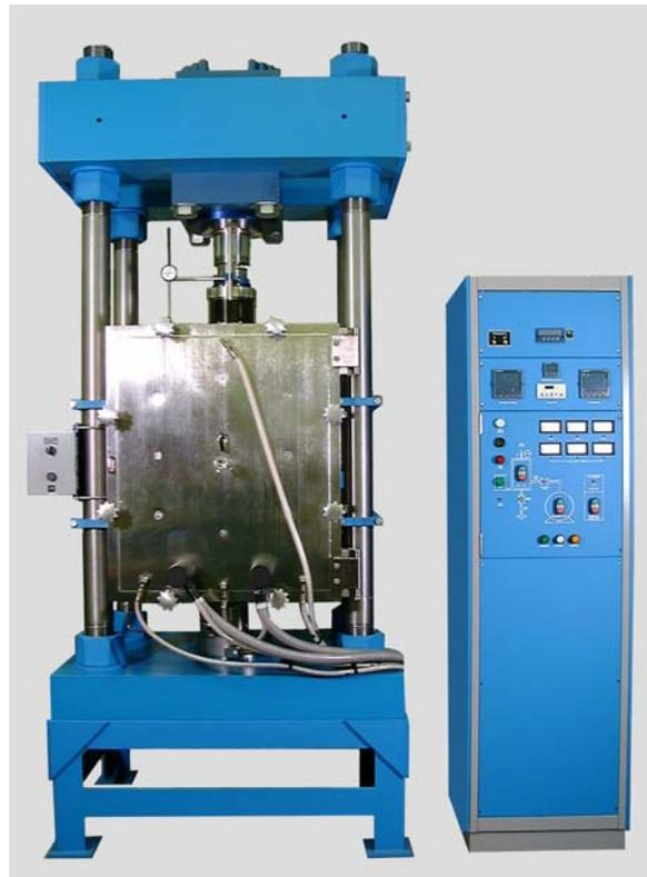
The hot press can be rated up to a maximum operating temperature of 2500°C (4532°F) and will operate in vacuum, inert atmospheres, Nitrogen and Hydrogen.
